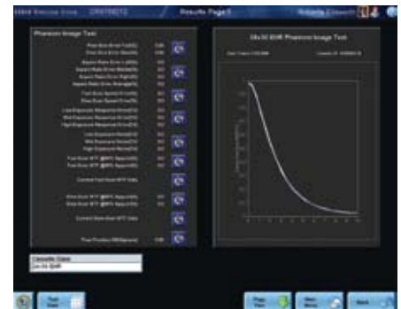
This graph shows the MTF response as a function of frequency (cycles/mm).
