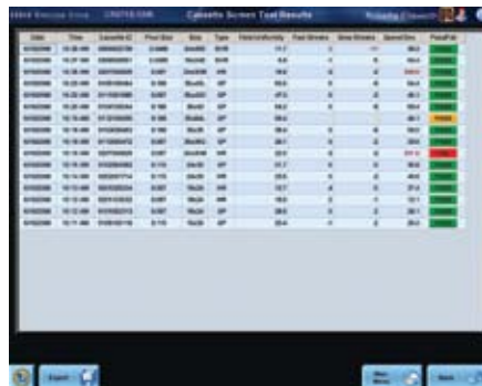
Test results data page displays a summary of up to 13 of the most recent test results for the different cassette sizes and types.
