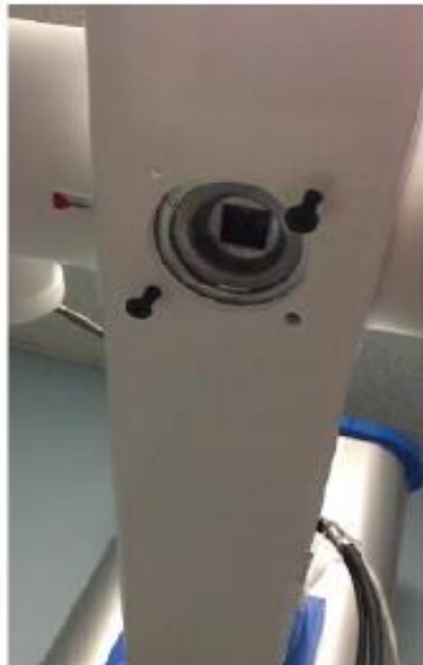
Figure 8: showing the 4 mounting holes at the bottom of the arm to mount the tube and the collimator ring
