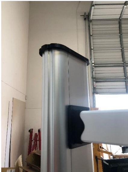
Figure 6: placing the top column cap
